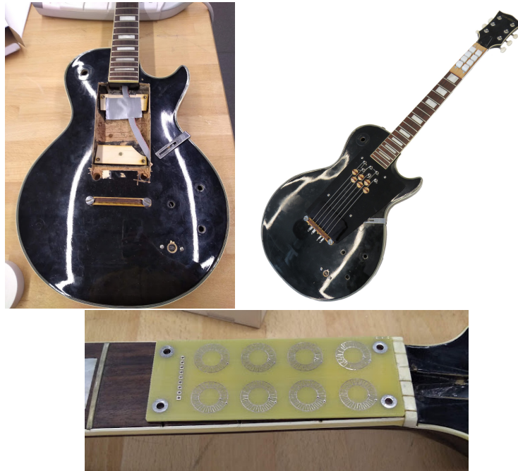
Figure 4. L: Les Paul body with material removed for electronics. R: completed S3 instrument. Bottom: custom PCB made to fit neck width
