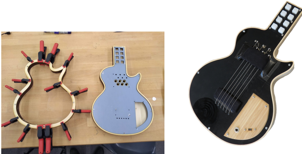
Figure 3. L: build process of S2 instrument using layers of glued plywood. R: finished S2 instrument Figure 3 Alt text: The image on the right shows the finished version of an instrument which resembles a smaller Les Paul-style guitar, but with a shorter neck embedded with eight white buttons in two rows of four. The image on the left shows the same instrument but with no buttons or strings attached, and some pieces of plywood that have been cut out in the shape of a Les Paul being clamped together while glue is drying. Figure 3 Long description: The left picture shows a top view of the outline of a Les Paul guitar-shaped body made out of plywood, held together with clamps. A piece of acrylic is next to it, which has been cut out to resemble the top of a Les Paul guitar but with a shorter neck. The neck has eight holes cut out. The right picture shows the finished instrument, which resembles a smaller Les Paul guitar with short lengths of string and eight white buttons. A wooden pick guard has a USB port and a jack cable input.
