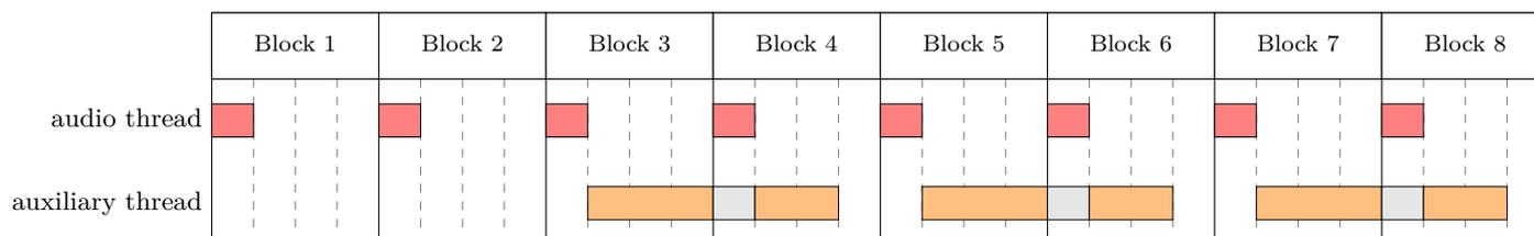
**Figure 5: Multi-threading.** The audio thread (highest priority) and the auxiliary thread are shown, respectively, in red and orange. Grey indicates that the thread is sleeping. In this example, the auxiliary thread waits for a buffer of two blocks of samples to be filled. For this reason, the auxiliary thread does not run in the first two blocks.
