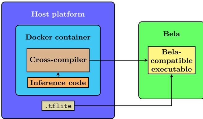
**Figure 4: Cross-compilation for Bela.** The inference source code is compiled in a Docker container in the host machine (e.g. a laptop). Both the Bela-compatible executable and the .tflite model are then transferred to the Bela.
