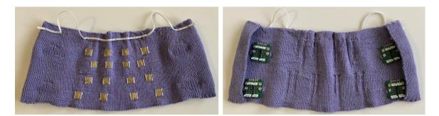
Figure 7.21: Amendments made to the collar: additional elastic is added to the inside of the collar to hold it up around the chin and provide support with straps around the ears (left). The excess fabric is folded over on the back to ensure a tight fit (right); these ends will be joined once the collar is on the wearer.
