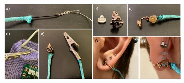
Figure 7.20: The construction of the earring reference electrode, starting with the cabling (a), stitching the conductive fabric to the earring pad (b-c), and securing the electrode to the collar and reference inputs (d) for a complete wearable (e). I wear the electrode along with my normal jewelry (f, g).
