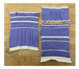
Figure 7.13: Samples of different rib structures added to the full-knit to provide indication of electrode sites.
