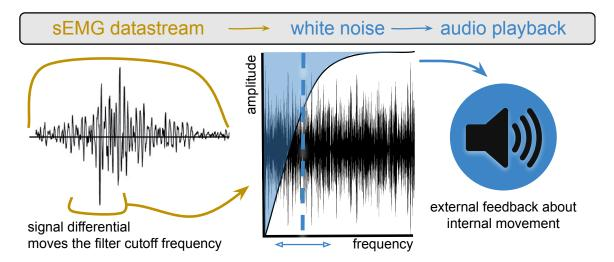
Figure 9.4: Translating the vocalist's sEMG signals to audio feedback: the differential of the sEMG signal is used to move the cutoff frequency of a filtered white noise. This audio is played back to the vocalist as an external feedback about their internal movement.
