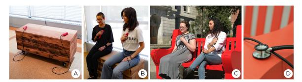
Figure 6.4: The Heart Sounds Bench (a,c) allows one or two people to sit together (b,c) and, with the help of stethoscopes connected to the inside of the bench (d), listen to a sonification of their heartbeats (Howell et al., 2019). Photos used with permission of Howell et al.
