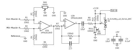
Figure 7.5: Version 3: The currently used circuit used for the VoxEMG, which also replaced the TL072 with the OPA1612. It is important in reproduction of this circuit that high-precision (ideally 0.1%) metal film resistors be used for R1-R4 to ensure the resistance in series with both electrodes is the exactly the same.
