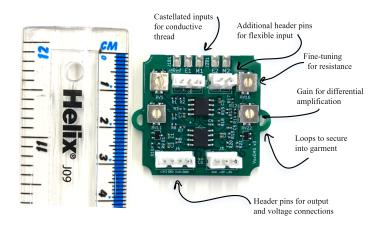
Figure 7.17: The VoxEMG board and some of its features for precision tuning and flexible I/O for wearable integration.
