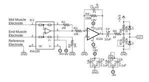
Figure 7.3: Version 1: The original circuit for sEMG signal acquisition and preamplifier schematic using three electrodes.
