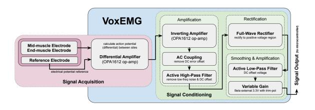
Figure 7.6: Signal flow through the VoxEMG board (Version 3 of the vocal sEMG circuit designed in this thesis).
