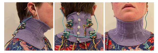
Figure 7.22: Wearing the completed knit collar, showing the knit's form on the neck compared to the original sEMG setup.
