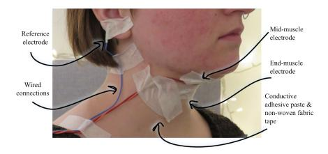
Figure 7.9: A photo of myself wearing the typical sEMG setup, with lots of fabric tape being used (even here, one can see the fabric tape by the labeled mid-muscle electrode is starting to peel off).
