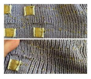
Figure 7.19: The conductive thread stitched along the knit (top). When stretched, the conductive traces stretch with the knit (bottom).
