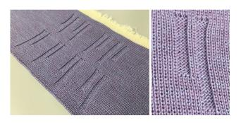
Figure 7.14: The ribbing added to the collar body; the relief stripes' end points provide visual and tactile representation of the electrode positions.
