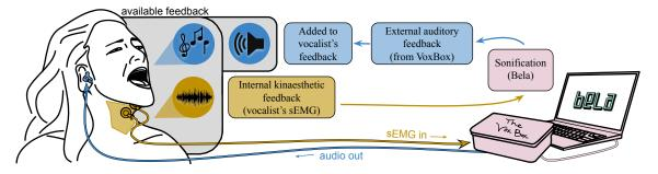
Figure 9.2: Using the VoxBox to externalise internal sensory experiences: the vocalist's internal laryngeal movements (internal kinaesthetic feedback, yellow) are captured with surface electromyography. The sEMG data is used by the VoxBox to generate a sonification (external auditory feedback, blue), which is added to the vocalist's existing auditory feedback of their singing (grey box).
