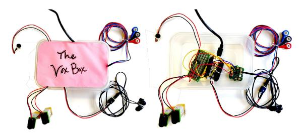
Figure 9.1: The VoxBox: external cables for electrodes, headphones, power supply (USB and 9 V batteries), and microphone (left), and internal VoxEMG, Bela Mini, and power routing (right).
