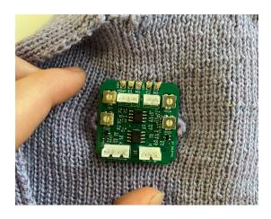
Figure 7.18: The VoxEMG board secured into the back of the collar.
