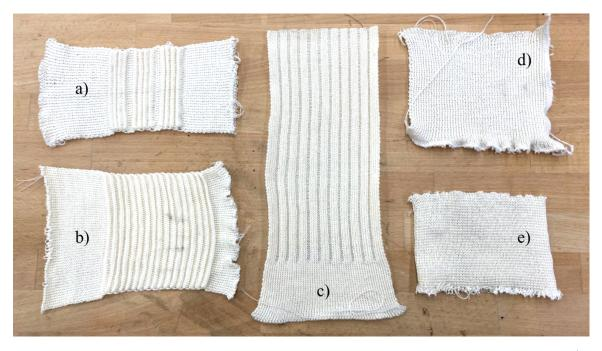
Figure 7.12: Samples of different knit structures for the collar body. Three Milano rib variations (a, b) were compared to a 2x3 rib (c) and two full bed rib stitches (d, e).
