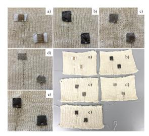
Figure 7.15: Swatches with stitched, soft fabric electrode probes for comparing materials. In order: a) silver-plated nylon zebra jersey, b) silver-plated jersey, c) tin-coated canopy mesh fabric, d) stainless steel mesh fabric, e) RayPad foam cushion.
