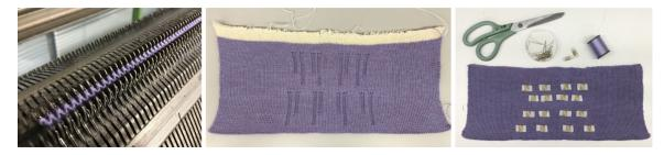
Figure 7.16: Creating the final collar body (left) and attaching the fabric electrodes (right). The final iteration uses the alternated relief stripes to mark the electrode locations externally (middle).
