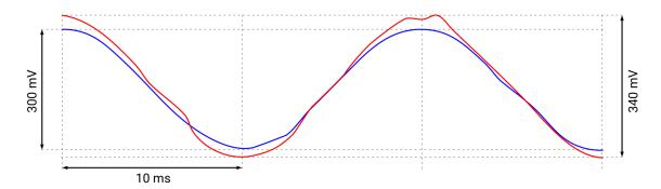
Figure 7.23: The vectorised signals from rigid electrode setup (red) and the fabric electrodes (blue) stitched into the collar. The signals measured are from the activation of the omohyoid during the singing exercise, as captured by the oscilloscope.
