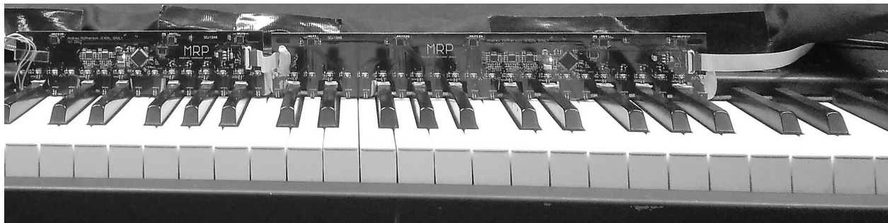
Figure 3. The keyboard scanner installed on the Yamaha CP-300.
