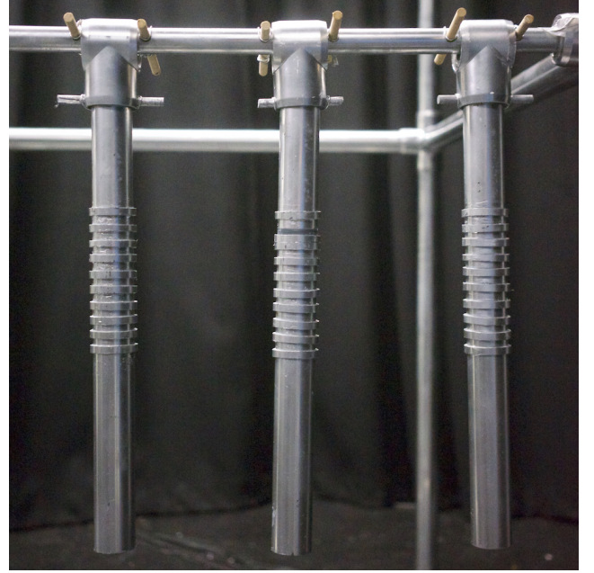
Figure 3: Close-up of pendulums, 50 centimetres long, with ten raised rings at one centimetre spacing.
