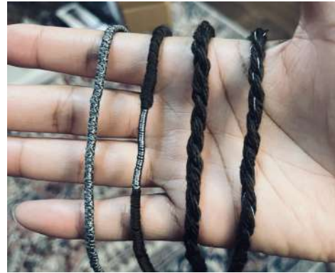
Figure 3: Chronological iteration of strand construction. From left to right: braided yarn wrapped with conductive thread; alternating conductive and non-conductive sections; roped yarn; and roped yarn interwoven with conductive thread.
