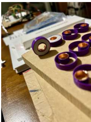
Figure 4: Early core prototype; this iteration includes a 3D-printed inner and outer core with the inner core being lined with copper tape.
