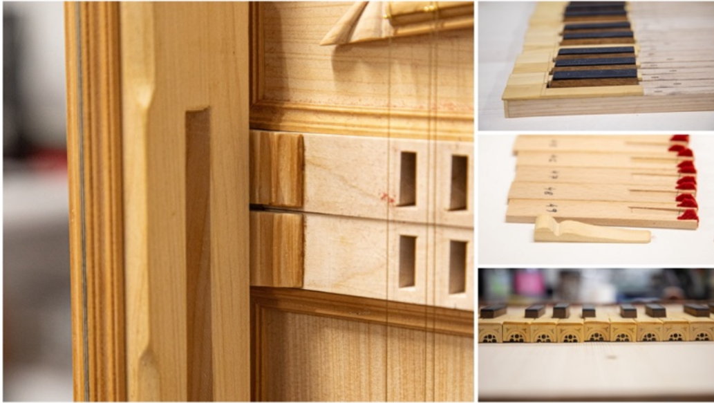
Figure 2: Details of the replica, including the key slots and sides, keys, and jacks with seagull plectra.
