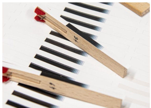
Figure 3: Gradient stickers applied to the side of the jack body. The coarse gradient scale was selected to maximise signal excursion while preserving signal readout stability.
