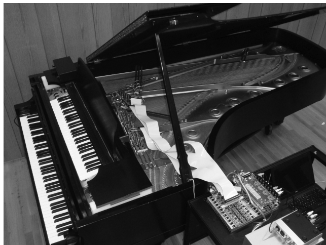
Fig. 4. Physical setup of the magnetic resonator piano in a Steinway D concert grand.
