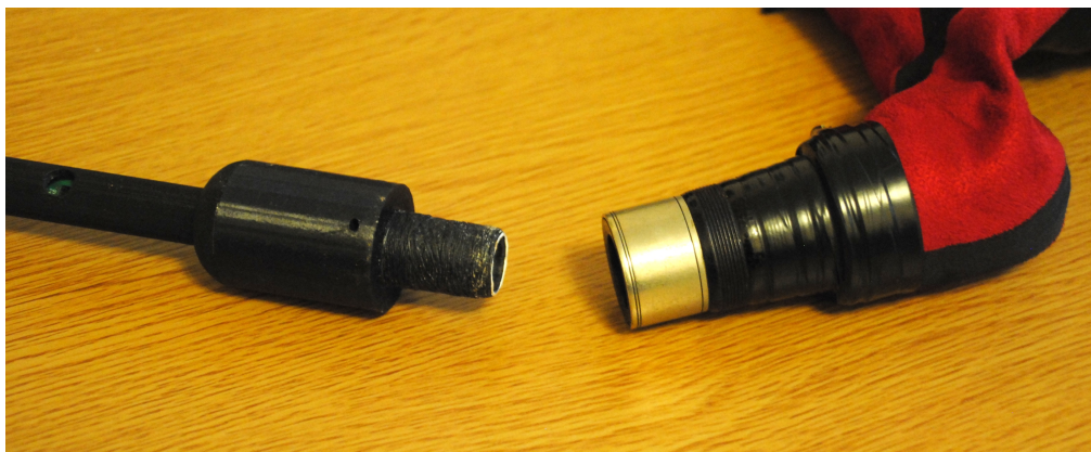
Figure 3.14: Top of digital chanter showing stock for insertion into acoustic GHB.
