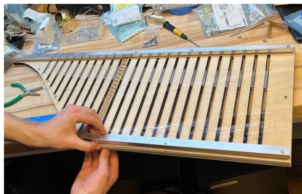
Figure 12: Laser-cut Magnet Rail
