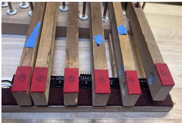
Figure 14: View of optical array from behind the manual – the rightmost key is depressed from the player’s position
