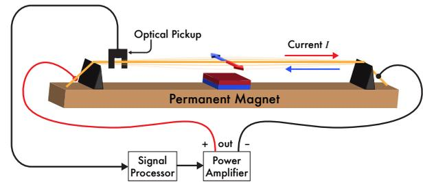
**Figure 5: Example of a Lorentz Force Feedback Sustainer system**
