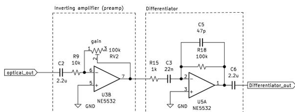
Figure 10: An op-amp preamplifier and differentiator
