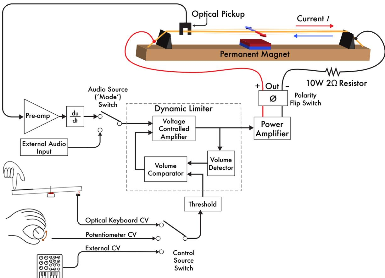
Figure 7: Full system diagram for one string of the Sparksichord
