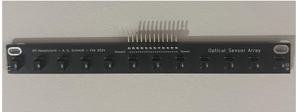
Figure 13: Optical Key Sensor Schematic & 12-channel optical keyboard sensor
