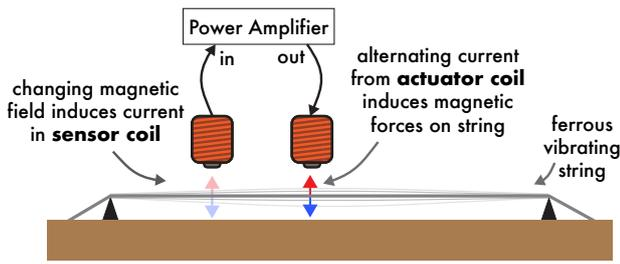
Figure 2: Simplified block diagram of EM Coil Sustaining, as is done in eBows
