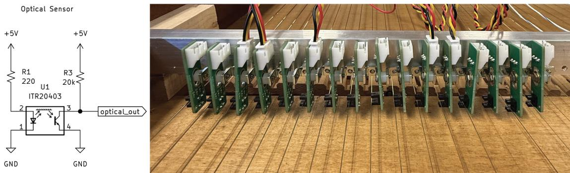
Figure 9: Optical String Sensor Schematic & the array mounted above strings
