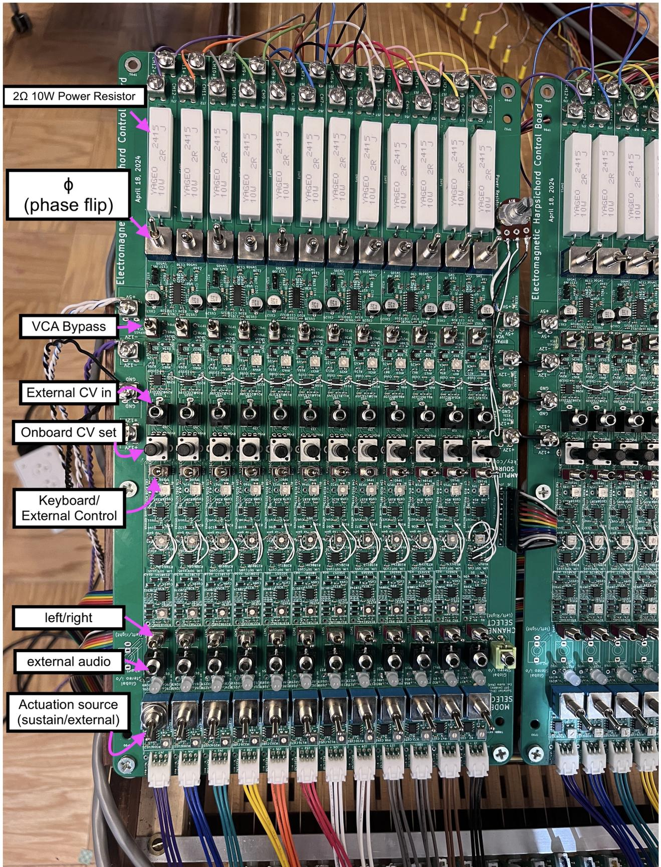
Figure 8: 12-channel Sustainer Board and its controls
