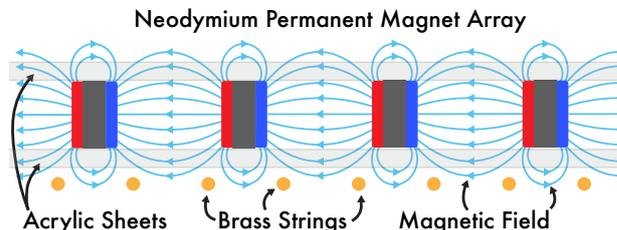
Figure 11: Side view of magnets and strings (where strings are going into the page)
