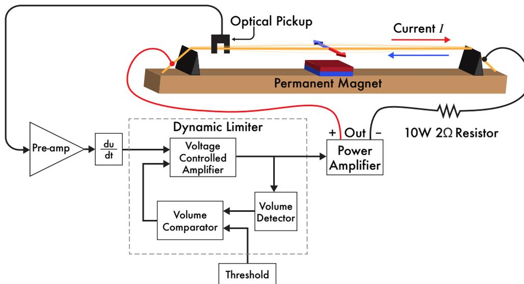
Figure 6: Lorentz Force string sustainer with differentiation and dynamically-controllable amplitude
