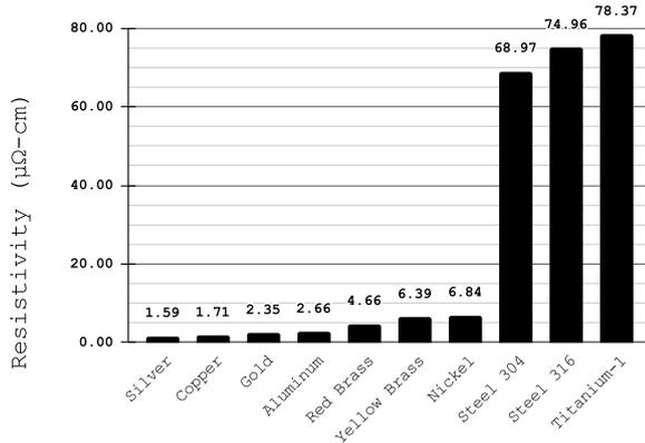
**Figure 4: Resistivity of conductive materials used in musical instrument strings (as reported by the CSNDT dataset by Eddy Current Technology Incorporated)**
