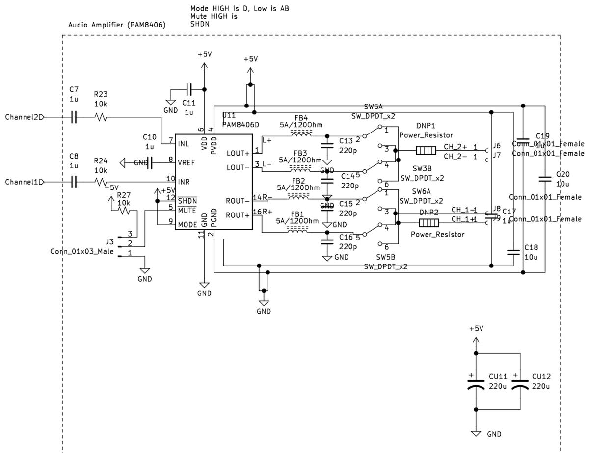
Figure 16: Circuit Configuration for PAM8406
